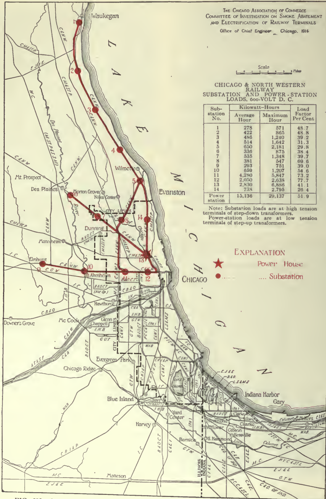
FIG. 623. LOCATIONS OF POWER STATION AND SUBSTATIONS FOR THE CHICAGO & NORTH WESTERN RAILWAY FOR THE 600-VOLT D. C. SYSTEM
